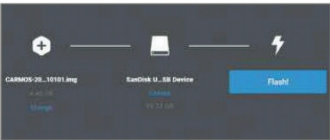
Etcher formats your USB stick, makes it bootable and installs the Chromium OS
